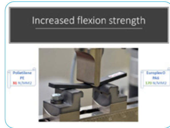
Fig 12.1 Polyamide 5 times stronger than polyethylene
